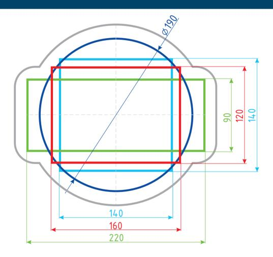
The above diagram is understood as exemplary dimensions of profiles which can be manufactured in Final S.A. However, all the queries are considered individually and there can be exceptions from this rule. Values in the above diagram are given in millimeters (mm).
