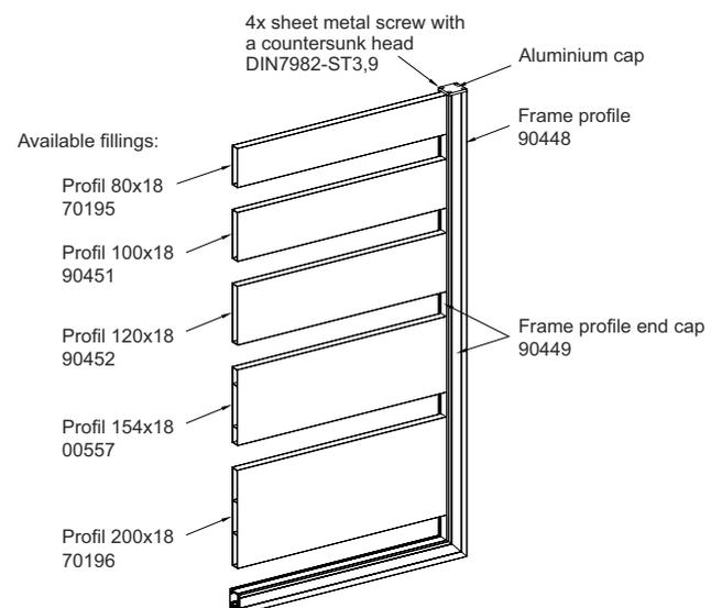
For assembly of the infill, use self-tapping sheet metal screws DIN 7981 or DIN 7504N: ST3.9 or ST4.2 (max. screw head height: 3.1 mm).
